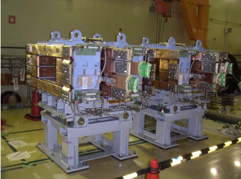
Injection bump magnet
