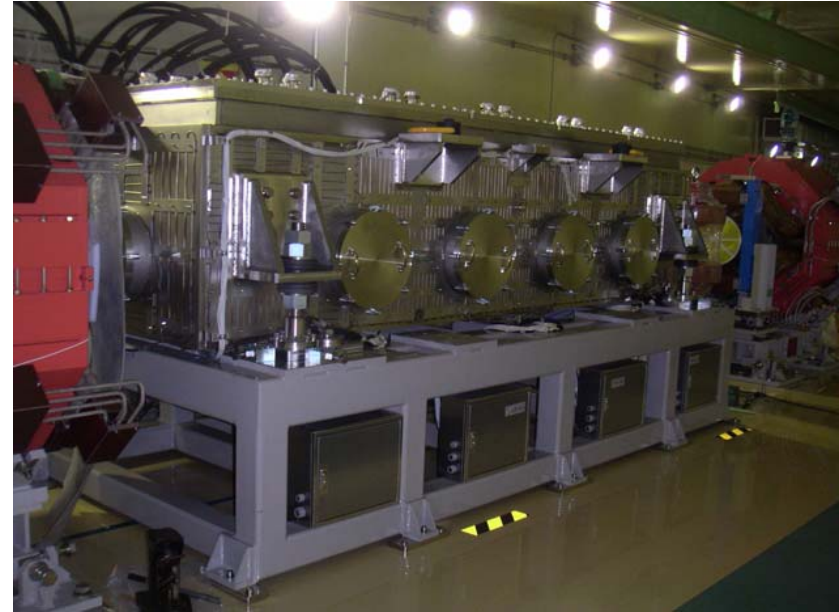
Extraction kicker chamber (5 kickers)
