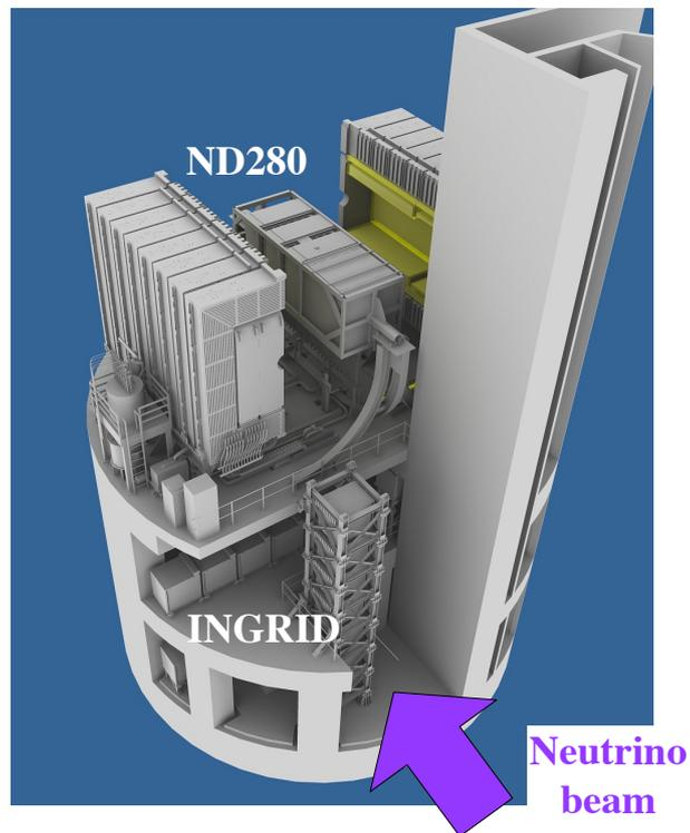
Figure 2.15: T2K near neutrino detectors. The ND280 detector and the magnet are located at the upper level, and the vertical and horizontal INGRID modules are located at the middle and bottom levels. The magnet is opened in this figure, though it is operated with its close position.
