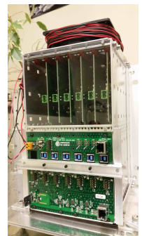
Figure 6: Left) Second version of the electronics readout Front End Board (FEBv2), received at the University of Geneva in March 2017. Middle) FEBv2 in minicrate. Right) rear of minicrate with 6 FEBs connected through a Backplane PCB on the lower half of the minicrate.
