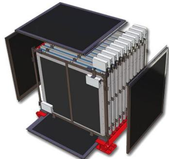
INGRID “cross” is formed with 14 identical modules + 2 diagonal modules made of plastic scintillator planes and iron targets surrounded by VETO planes.
