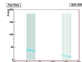
Background: Muon from the  $\nu$  interaction at the upstream wall. Rejected by fiducial volume cut.
