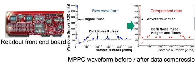
MPPC waveform before / after data compression
