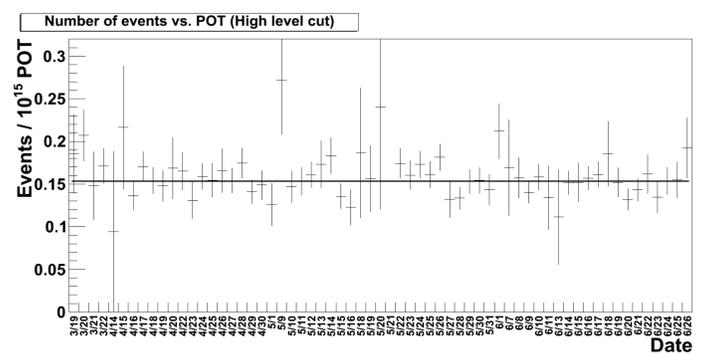
As a result, we confirmed that the FGD is observing neutrino events with stable rate. The measured event rate was 1.5 events / 10<sup>15</sup> POT (chi-square / ndf = 0.77). Systematic error for this number is not calculated yet, but this number roughly agree with the expected event rate in MC.
