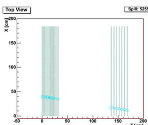
Background: Muon from the  $\nu$  interaction at the upstream wall. Rejected by fiducial volume cut.
