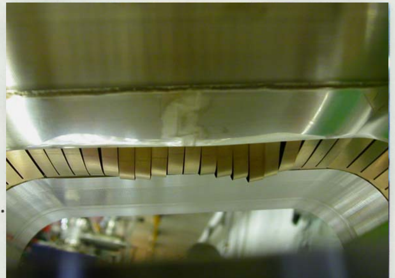
Thermal deformation of the fingers for rf shield of bellows.
