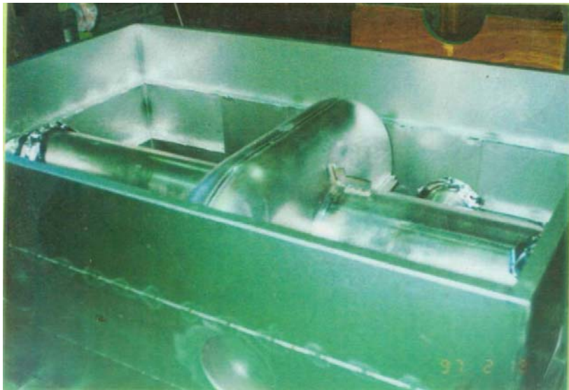
Annealing at 700°C for 3 hours
