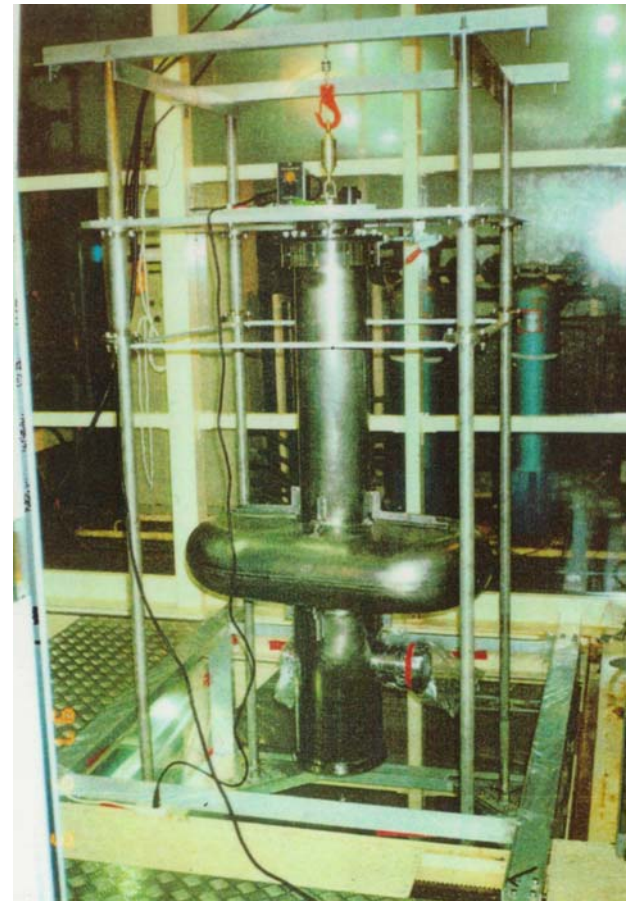
High Pressure Water Rinsing by 80 bar Ultra-Pure water
