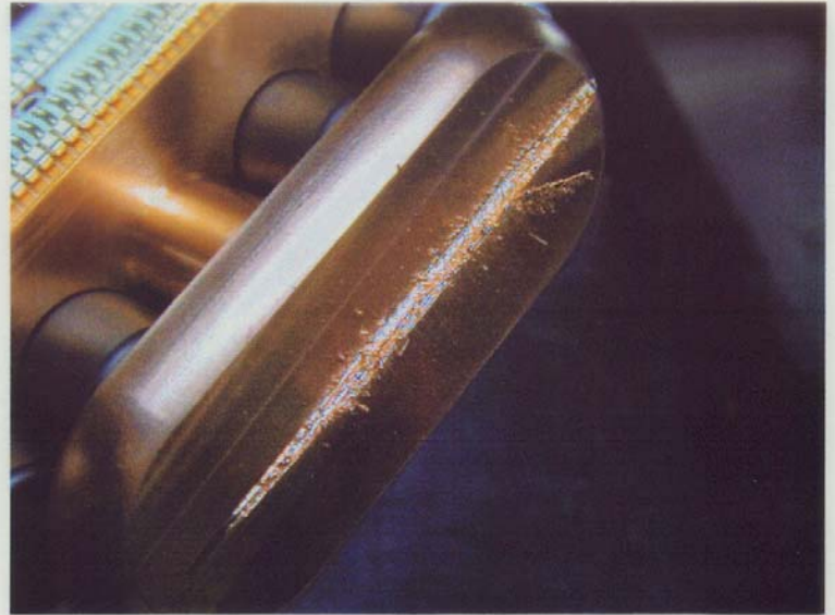
Heavy groove on the surface of a copper movable mask in HER.
